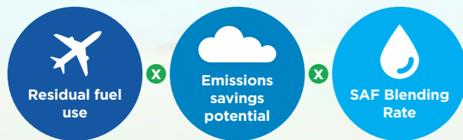
Figure 14: The three key components that determine the emissions abatement potential of SAF.
